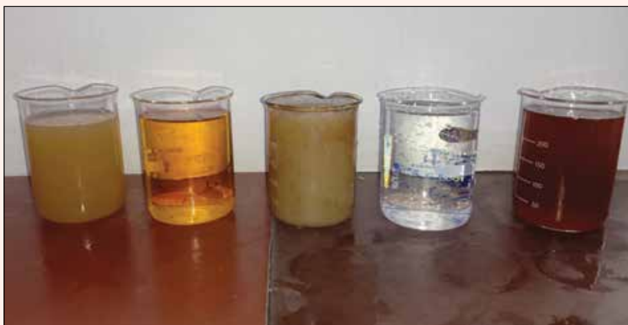
Ultrafiltration + Nano Filtration of Alkali Extraction stream.
