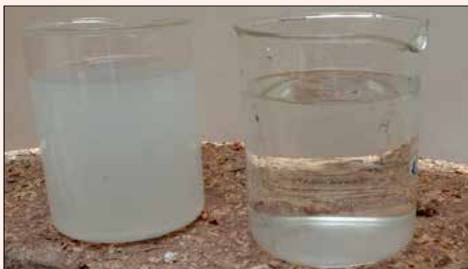
Save-all outlet from paper machine and feed to ultrafiltration (left) and filtrate (permeate) of ultra-filtration (right).
