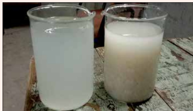
Paper machine back water fed to UF and reject to be recycled back in wet end operations.
